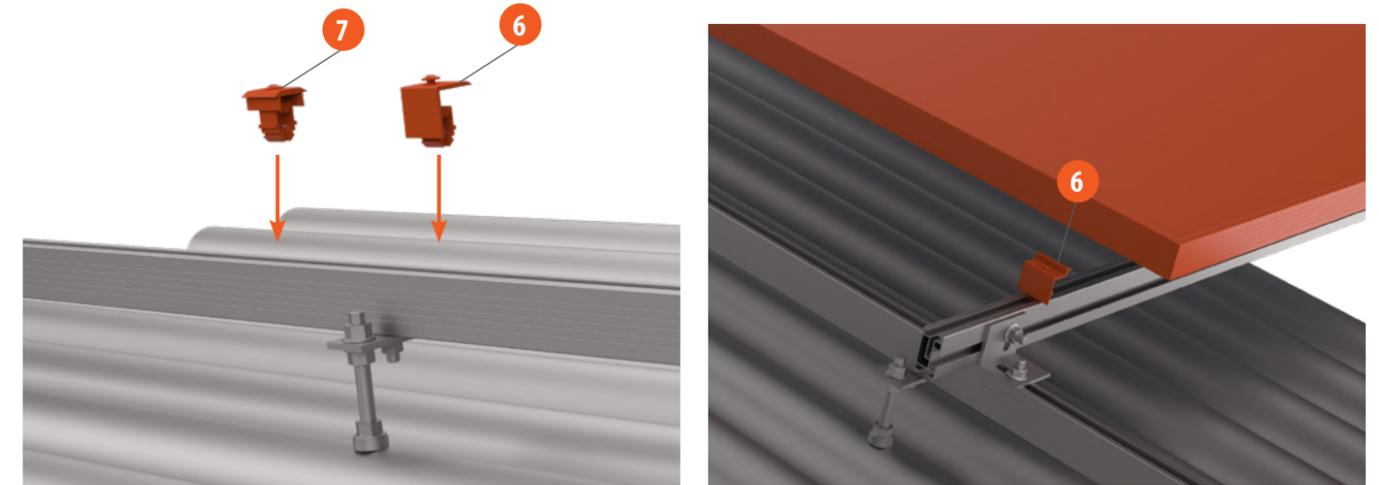
Insert the lower part of the end or middle clamp into the top slot of the EasyMount™ 48 profile and rotate by 90°. Lay the PV modules on the profiles and fix them with the clamps using electrical drill and bolt socket applying a torque of maximum 10 Nm. Each module has to be fixed by four clamps. The end clamps are used at the ends of each row, while the middle clamps are used to fixate two adjoining modules in the same row. All clamps are delivered preassembled.
