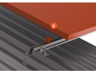
Insert the lower part of the end or middle clamp into the top slot of the EasyMount™ 48 profile and rotate by 90°. Lay the PV modules on the profiles and fix them with the clamps using electrical drill and bolt socket applying a torque of maximum 10 Nm. Each module has to be fixed by four clamps. The end clamps are used at the ends of each row, while the middle clamps are used to fixate two adjoining modules in the same row. All clamps are delivered preassembled.
