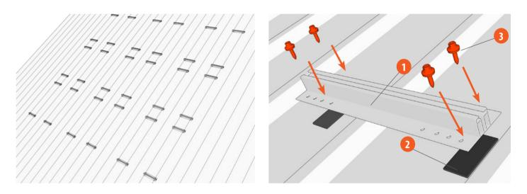
Stick 2 pieces of the self-adhesive protective EPDM rubber on the previously calculated spots. Place the rail above it and fix it by driving in 4 screws. Repeat until all the needed rails are installed.
