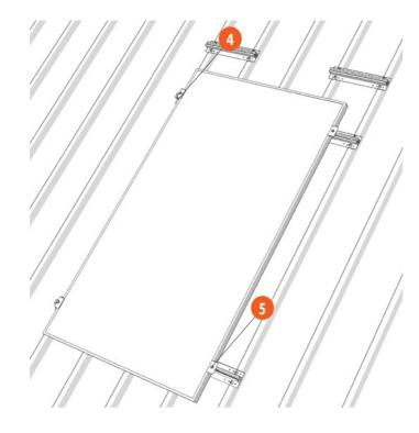
Maximum continuous length of a single block (vertical or horizontal) is 20 m. After this length, a space of at least 50 mm between the rails for thermal separation must be added.
