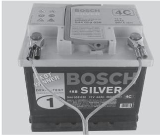
Using terminal clip attaching to car battery
