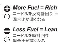
If idle is unstable, adjust the low speed needle to get a stable idle. Afterwards, you need to readjust the idle adjustment screw.
