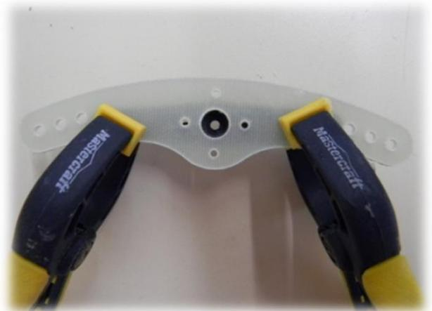
**40-) Secure your arm underneath the composite arm, making sure that both center holes are in line.**
