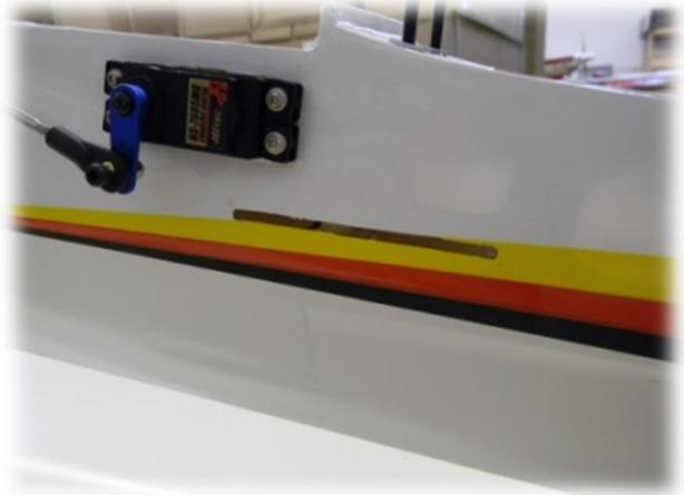
**38-) Left side. Go around any covering openings with a "covering iron" to prevent the covering from peeling off.**
