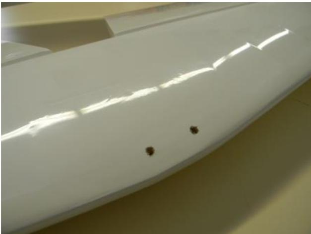
**19-) On the top and bottom (front section) of the stab, locate the two small holes. Remove the covering to expose the holes.**
