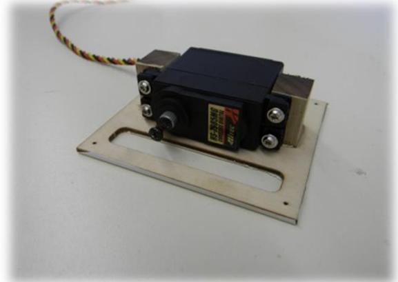
**64-) Secure one servo on the cover with four servo screws.**
