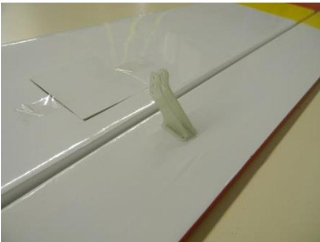
**15-) Repeat the horn assembly procedure for both ailerons.**
