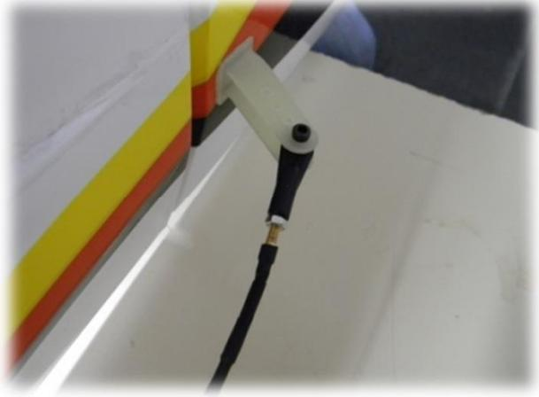
**46-) Secure the pre-assembled cable ends to the rudder horn.**
