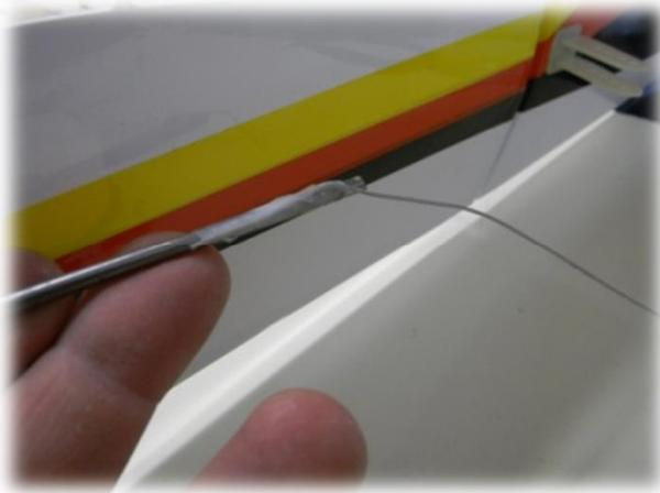
**45-) A simple trick to "fish-in" the pull-pull cables is to use a small diameter pushrod and "tape" one end of one of the cables. Then, pull the cables in.**
