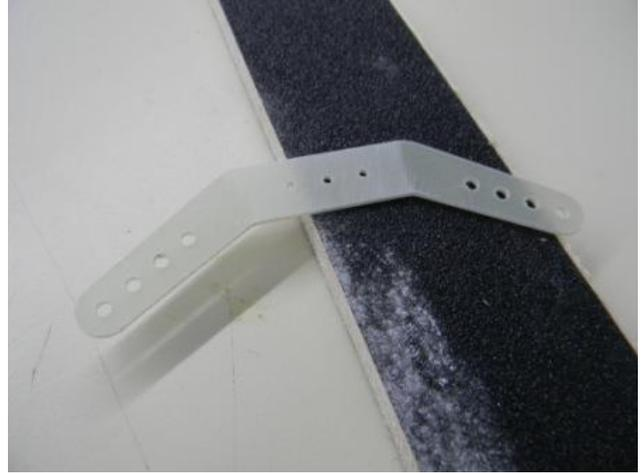
**10-) Sand the two rudder horns (center-section only) and clean with alcohol.**
