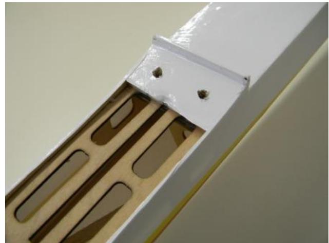
**20-) Do the same on the front of the stab fuselage saddle section to expose the pre-installed blind-nuts.**
