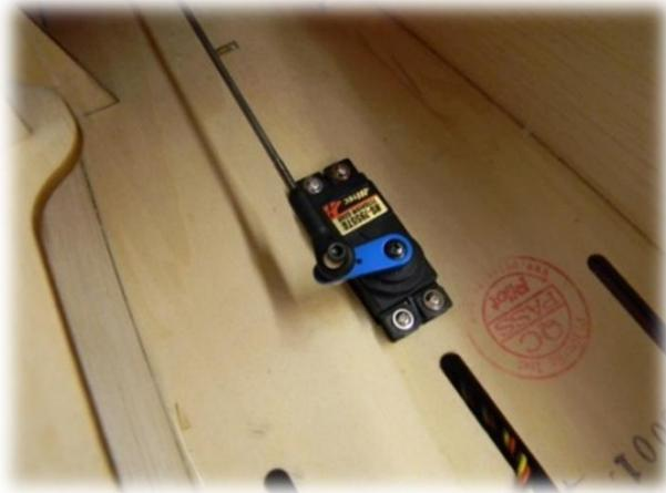
**50-) Look for a pushrod with one ball link on one end only. Attach it to this servo. This pushrod will exit from the nose and will secure the towing cable to your glider (see next two pictures)**
