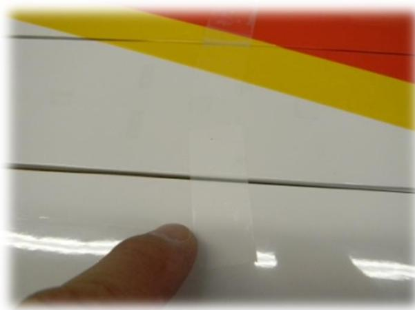
**52-) Also place a strip of masking tape in the middle of the spoilers (important)**
