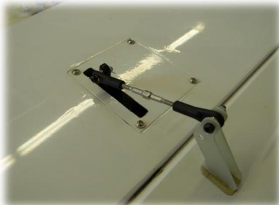
**65-) The picture is self-explanatory. Secure the cover with the supplied wood screws.**
