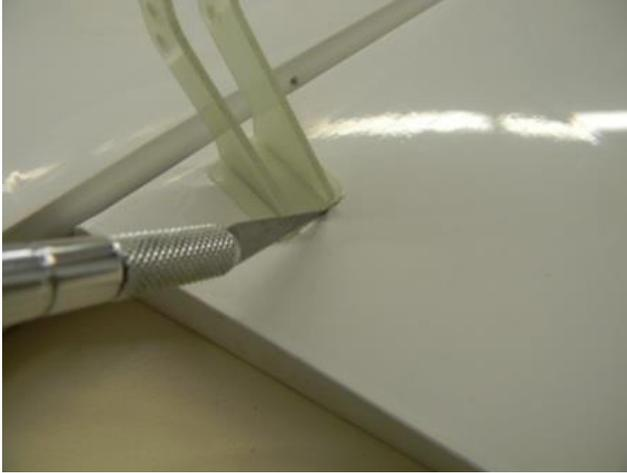
**5-) Insert the horn assembly into the Left elevator and cut the covering around the horn retainer.**
