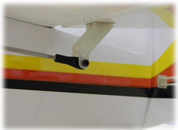
**34-) Attach the other end of the pushrods to the elevator horn. Use the supplied key to adjust the pushrod mechanically.**
