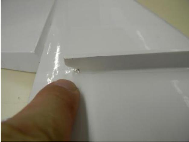
**21-) Underneath the stab, at the rear section, notice the small notch.**
