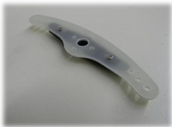
**42-) Drill two holes (more/depending of your servo arm choice) and insert some of the supplied small screws.**
