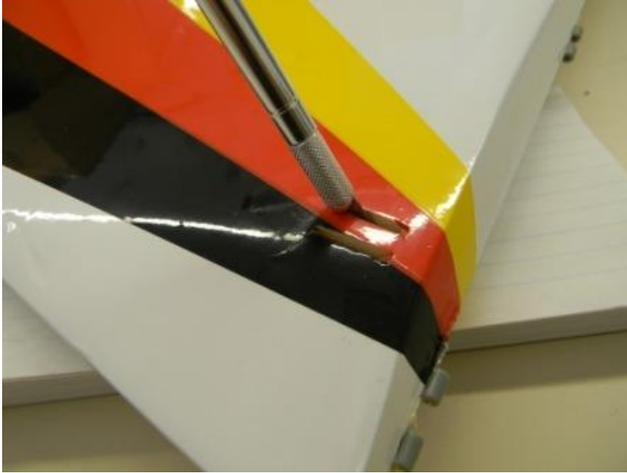
**9-) Locate the rudder and repeat the same process as the elevator to open the cavity for the rudder horn.**
