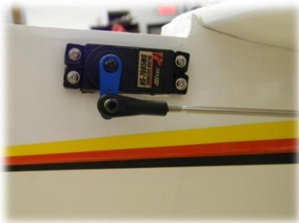
**33-) Secure the stab to the fuselage. Plug your elevator servo in your receiver and center it. Attach the supplied elevator pushrod to the servo arm. That pushrod has two ball-links factory installed onto it.**
