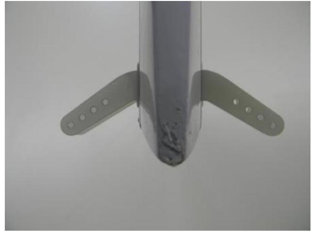
**14-) Position the second horn retainer with epoxy and adjust both horns so that they properly match.**
