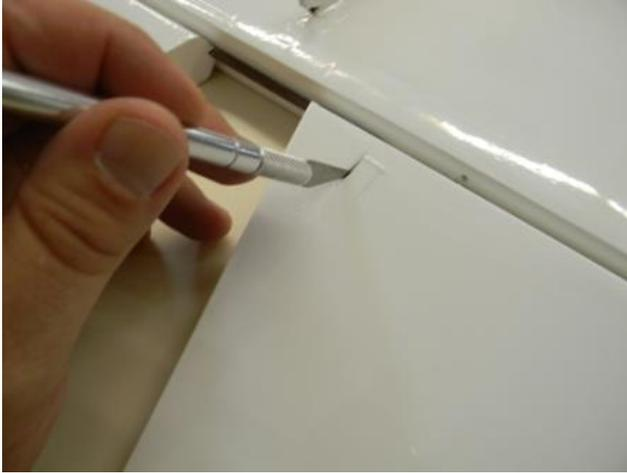
**1-) Locate the stab/elevator assembly. From the bottom Left side, cut into the covering, exposing both pre-cut slots.**
