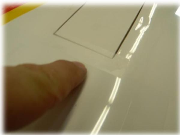
**51-) Wing spoilers. Temporarily secure the spoilers in place on the wing panels using masking tape at both ends of each spoilers.**
