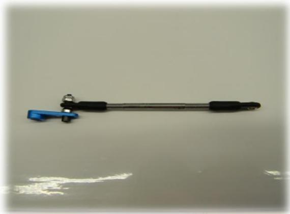
**59-) Prepare a 3 1/4" (82mm) long pushrod and put one ball link at each ends.**
