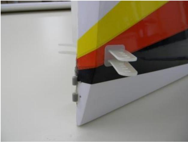
**13-) Like the elevator, apply epoxy to the horn assembly and insert into position.**
