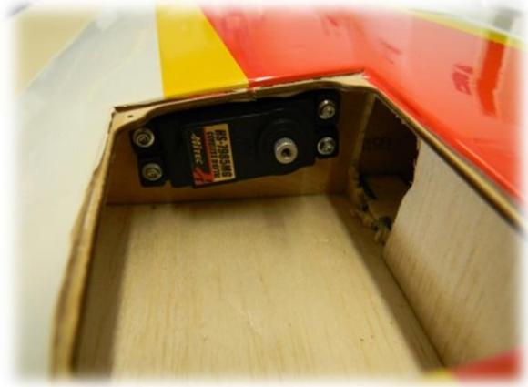
**58-) Position the servo exactly as shown and secure with servo screws. A long screwdriver will work fine to secure the screws in place.**
