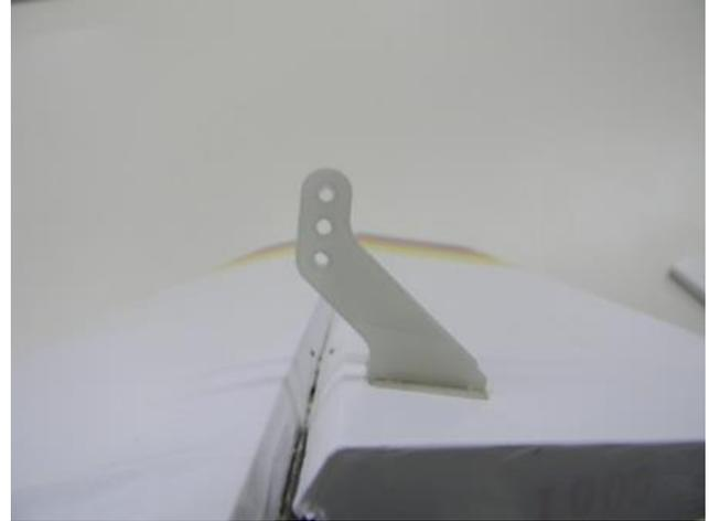
**8-) Align both horns so that the holes in both of them are parallel to each other. Let the epoxy cure. Repeat the same process for the Right elevator.**
