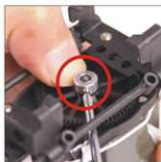
12. 齿轮固定环锁紧主齿轮 Lock up the main gear with the gear retainer ring.
