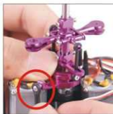
8. 伺服器摆臂上的拉杆头与倾斜盘连接 Connect the push-rod on the servo horn with the swashplate.
