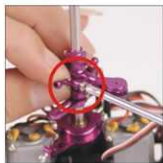
5. 夹头片装在下中心座组上并用螺丝锁紧 Install the grip set onto the bottom central holder set and lock it up with the screws.
