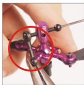
18. 单孔拉杆与主翼夹头连接 Connect the control link with the main blade grip set.
