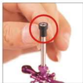
6. 固定环装上主轴 Install the retainer ring on the main axle.
