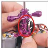
7. 双孔连杆连接倾斜盘与旋转夹头 Connect the swashplate and main blade grip set with the ring-like push-rod.
