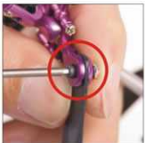
15. 主旋翼A装上夹头片并用螺丝锁紧 Install the grip set on blade A and lock up with screws.
