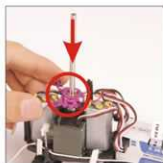
2. 将倾斜盘装入主轴 Install the swashplate on the main axle.
