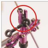
16. 稳定锤装上中心座组 Install the stabilizer set on the central hub set.
