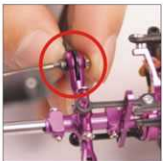
14. 主旋翼B装上夹头片并用螺丝锁紧 Install the grip set on blade B and lock up with screws.
