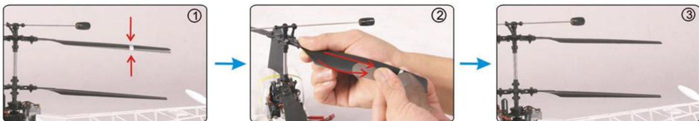
(1) 主旋翼旋转不在同一平面 Main blades don't rotate in one plane.
