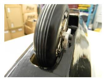
17-) Insert the screw from one side, slide on one spacer and the wheel.
