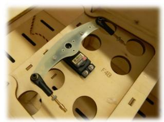
44-) Install your rudder servo, plug it into your receiver and center it. Secure the rudder servo arm assembly. Locate the pull-pull cables. Two of the ball links are not crimped on the cables. Remove them and screw them to the rudder arm as shown.
