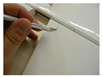
1-) Locate the stab/elevator assembly. From the bottom <u>Left side</u>, cut into the covering, exposing both pre-cut slots.
