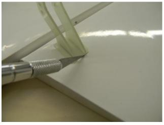
5-) Insert the horn assembly into the Left elevator and cut the covering around the horn retainer.
