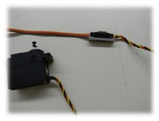
29-) The elevator servo requires a 48" (121cm) servo lead extension. Secure both the servo and the extension with one of the supplied Grey safety clips.
