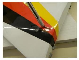
9-) Locate the rudder and repeat the same process as the elevator to open the cavity for the rudder horn.
