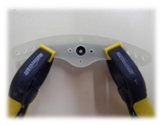
40-) Secure your arm underneath the composite arm, making sure that both center holes are in line.
