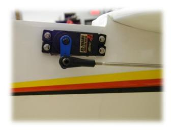
33-) Secure the stab to the fuselage. Plug your elevator servo in your receiver and center it. Attach the supplied elevator pushrod to the servo arm. That pushrod as two ball-links factory installed onto it.
