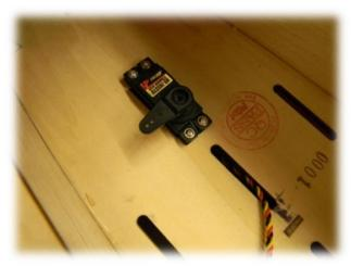
49-) In the cockpit, front section, there is a cavity for the "tow release system". Install a servo in that cavity.
