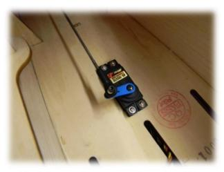
50-) Look for a pushrod with one ball link on one end only. Attach it to this servo. This pushrod will exit from the nose and will secure the towing cable to your glider (see next two pictures)
