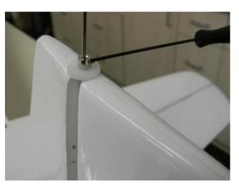
26-) From the top, slide the plastic round disc and secure it with the small wheel collar.
