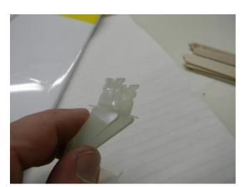
7-) Also apply epoxy on the horn assembly, where it will fit into the elevator.
