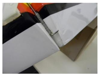
25-) Push the steel wire until it reaches the bottom hinge as shown.
