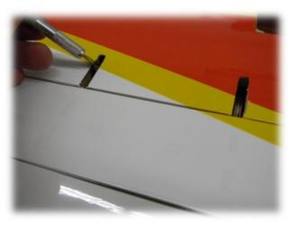
56-) Remove the masking tape. Using your finger, locate the three slots in the wing, in front of the spoilers. Once located, cut the covering to allow the spoilers to move upwards.
