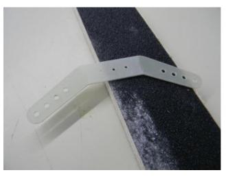
10-) Sand the two rudder horns (center-section only) and clean with alcohol.
