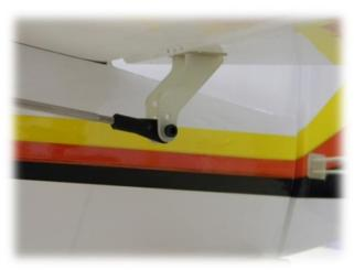
34-) Attach the other end of the pushrods to the elevator horn. Use the supplied key to adjust the pushrod mechanically.
