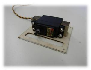
64-) Secure one servo on the cover with four servo screws.
