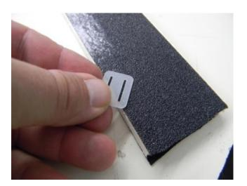
3-) Sand one side only of the horn retainer as shown. The sanded side will face on the elevator surface.
