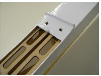
the stab fuselage saddle section to expose the pre-installed blindnuts.
