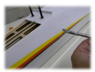
36-) Carefully seek the small cavity for the rudder pull-pull cables on both sides of the fuselage. Look at the picture carefully for reference. Use a knife to cut and remove the covering.
