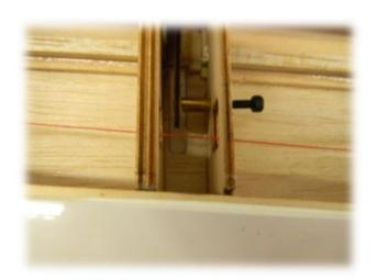
53-) Start with either tip spoiler hinges. Insert one Brass spacer using one of the M3 screws.
