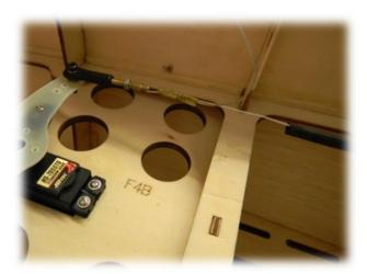
47-) Attach the other ends to the ball link connectors as shown and "crimp" the Brass retainers. NOTE: Crosse the cables in an "X" fashion inside the fuselage. This will provide a thither pull-pull cable set-up.
