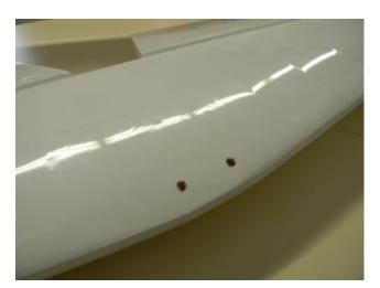
19-) On the top and bottom (front 20-) Do the same on the front of section) of the stab, locate the two small holes. Remove the covering to expose the holes.
