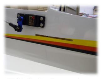
38-) Left side. Go around any covering openings with a "covering iron" to prevent the covering from peeling off.
