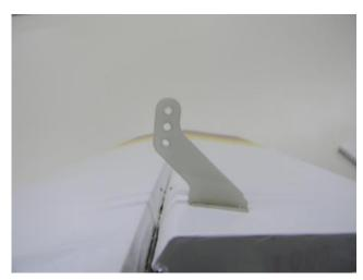
8-) Align both horns so that the holes in both of them are parallel to each other. Let the epoxy cure. Repeat the same process for the Right elevator.
