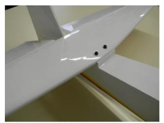
23-) Position the stab by sliding it into the inter-lock inside the fuselage and secure it with two 40mm screws and washers. Once positioned, glue the stab to the fuselage, after final assembly only.
