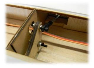
60-) Slide the pushrod from the bottom of the wing into the front servo cavity. Attach one end of the pushrod to the center spoiler rib as shown.
