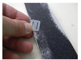
11-) Also sand the two rudder horn retainers (Left/Right) and clean with alcohol.
