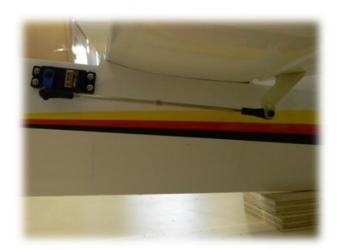
35-) Completed elevator assembly. Now, remove the stab for the next step. Repeat the process for the Right elevator servo.
