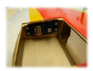
58-) Position the servo exactly as shown and secure with servo screws. A long screwdriver will work fine to secure the screws in place.
