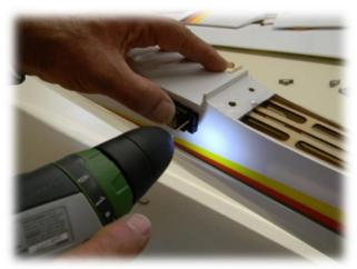
32-) Insert the elevator servo. Drill small pilot holes and secure with servo screws. NOTE: The front of the servo must go towards the front of the fuselage.
