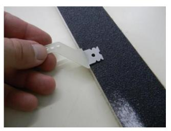
2-) Using a sanding bar, sand the top section of two supplied control horns on both sides and clean with alcohol.
