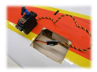
57-) Prepare the spoiler servo by attaching an appropriate servo lead extension and securing with a Grey safety clip. As for the elevator, you will find a Red string attached to the root rib and near the servo cavity to "fish-in" the servo lead extensions.
