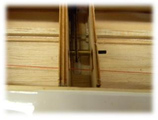
54-) Then, add another smaller Brass spacer as shown. You will need to "shave" the spacers for proper fitting between the spoiler hinges. Then, secure the screw with an M3 nut (Do not over thigh the nut)
