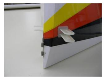
13-) Like the elevator, apply epoxy to the horn assembly and insert into position.
