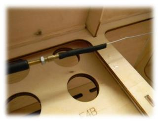
48-) Cut the remaining cable and slide over the heat-shrinkable tube over the Brass crimps. Using a heat-gun, shrink the tube as shown.
