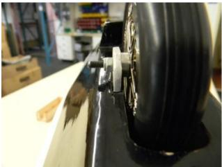
18-) on the other side, slide the other spacer, push in the screw and secure the screw using the **Nylon lock-nut.**
