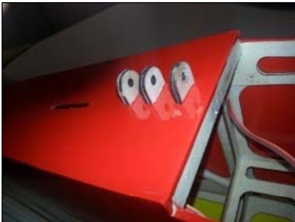
4-) While the epoxy is curing, insert the two parts F51 in the remaining two slots. Then, push in completely the Black tube.
