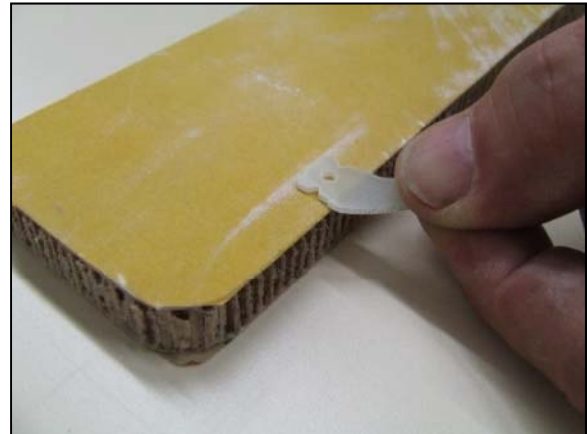
15-) Using a sanding bar, sand the horn section (on both sides) that will be inserted into the elevator for better glue adhesion.
