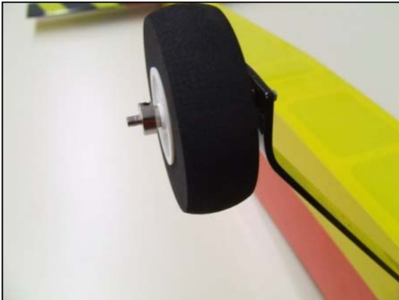
52-) Position the wheels and secure with another wheel collar.
