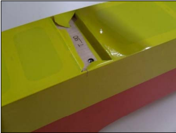
48-) Cut the covering from the first gear location (near the firewall)
