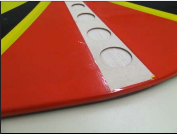
12-) Using a modeling knife, cut along the marked lines and remove the covering.
