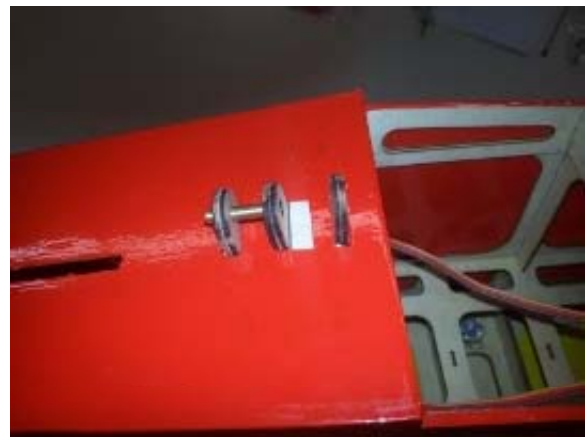
5-) Bond the Brass sleeve into both F51's as shown. Remove some small material in front of the first F51 to expose the wood.
