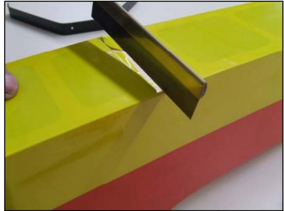
49-) Using a small saw, cut into both fuselage sides to clear the gear.
