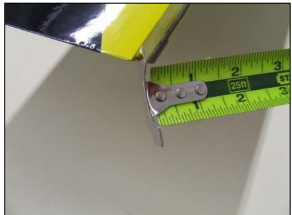
19-) Before the epoxy cures, align the stab by equally measuring from each wing tips as reference.
