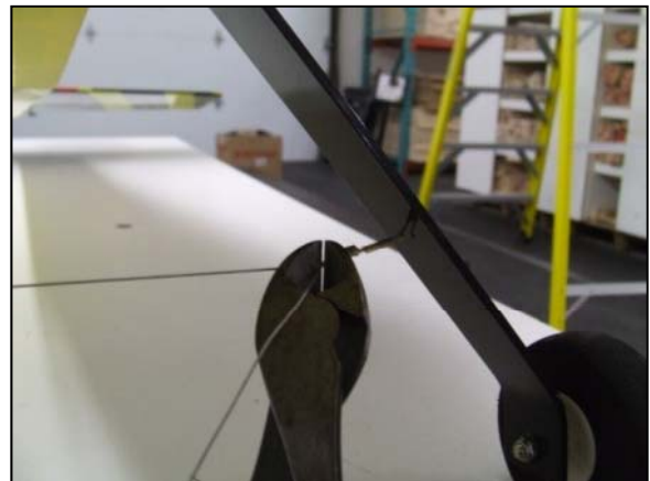
55-) Crimp the Brass sleeve against the steel cable and cut the remaining cable.
