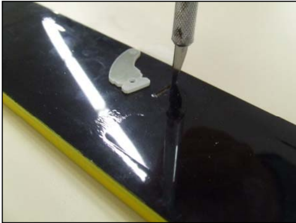
16-) Locate the pre-cut slot on the bottom of the elevator and cut to remove the covering.
