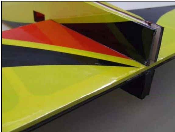
18-) Apply 30-minute epoxy to both the stab and fuselage sections and slide the stab into position.
