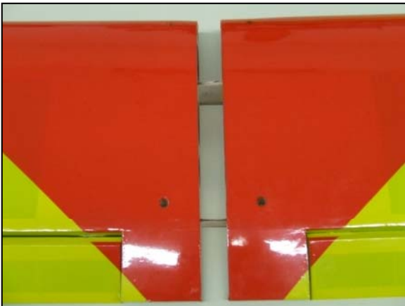
3-) Slide the other wing panel over the plywood joiners.
