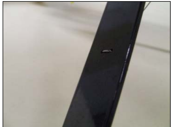
53-) Gear stiffening brace. There are two holes per gear sides, near the middle. Insert in a “U” shape the supplied steel cable from your hardware bag.
