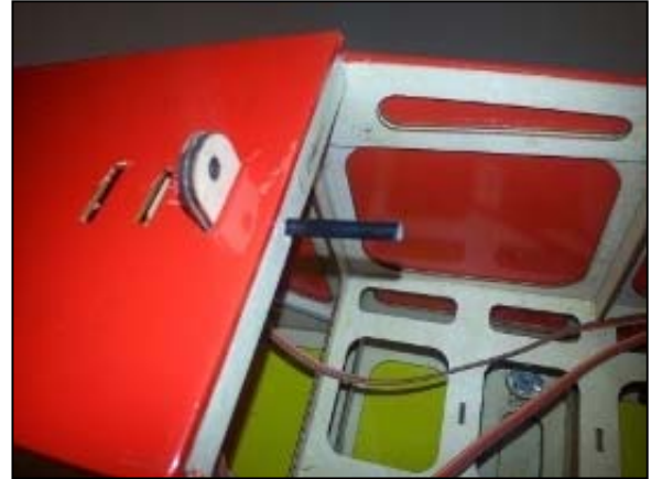
3-) Using 30-minute epoxy, slide into the fuselage part F51A and secure with the Black tube.
