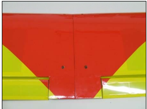
4-) Bring both wing panels together and verify for proper fit.
