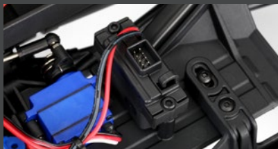
LED Lighting Module Installed
